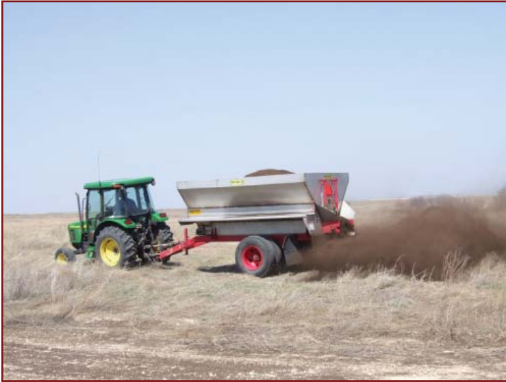
This broadcast application, utilizes a spinner unit, which projects compost from the rear of the spreader at a calibrated rate of 10 tons per acre.
