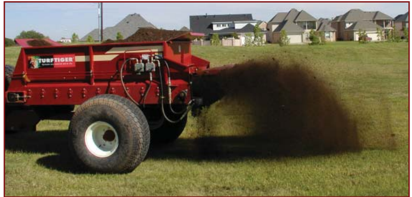
Turfgrass application units, like this one shown above, are extremely versatile and can accurately apply compost at varying rates.
