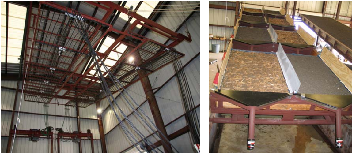
Figure 7. Oscillating rain rack with emitters (left) and non-vegetated treatment plots (right) hoisted under the rack at a 3:1 sideslope.
