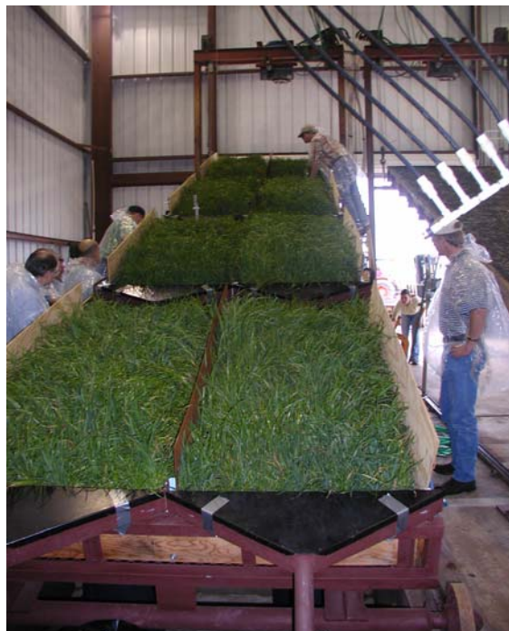
Figure 8. Rainfall simulation on vegetated ECC and IF treatment plots.
