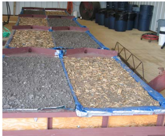
Figure 4. Metal bed plots with the IF treatment incorporated into soil and the ECC treatment applied on the soil surface.
