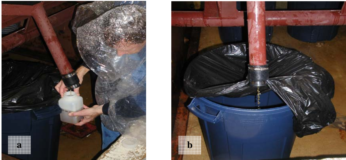
Figure 9. Samples of first flush (a) and subsequent runoff (b) being collected during rainfall simulation event.
