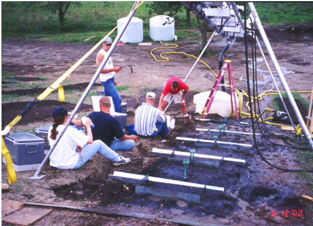
Figure 1. Rainfall simulator and test plot setup during interrill runoff sampling.
